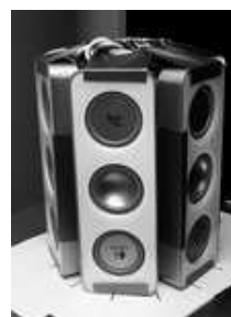
Fig. 8: Prototype loudspeaker array consisting of six Logitech Z4 loudspeakers arranged as a cylinder having a radius r \approx 8 cm.
